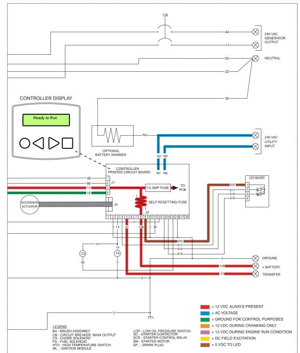
Figure 1. Circuit Condition - Utility Source Voltage Available
